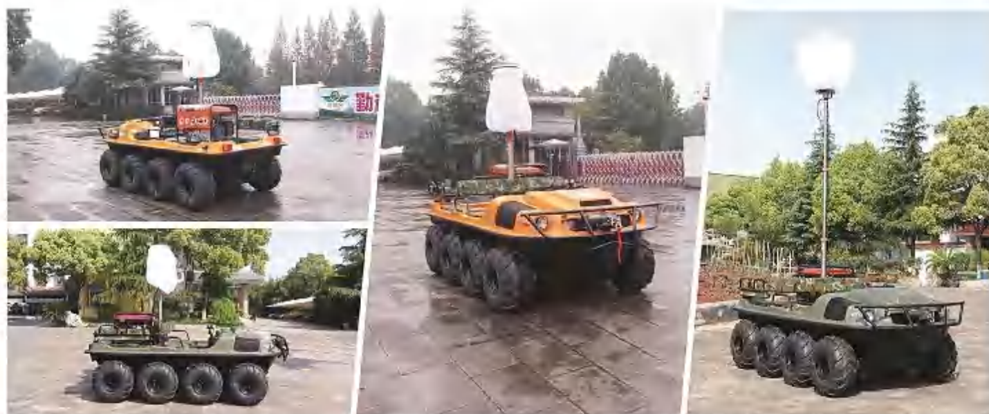
应急照明与供电 Emergency Lighting and Power Supply Device
